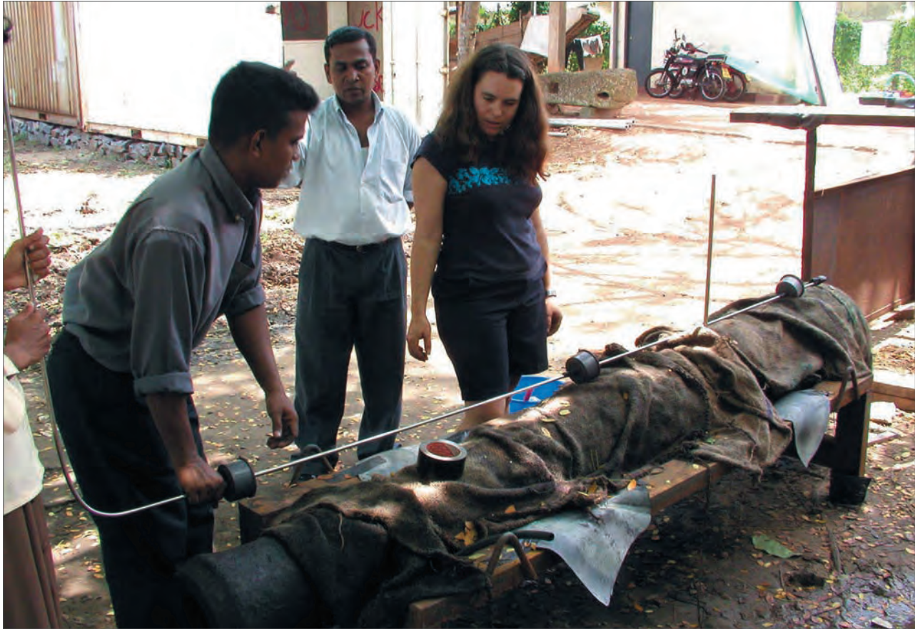
Figure 4.16 Placing the cannon on cradle and internal anodes for the electrolysis treatment of the cannon (02/GHL/175)
