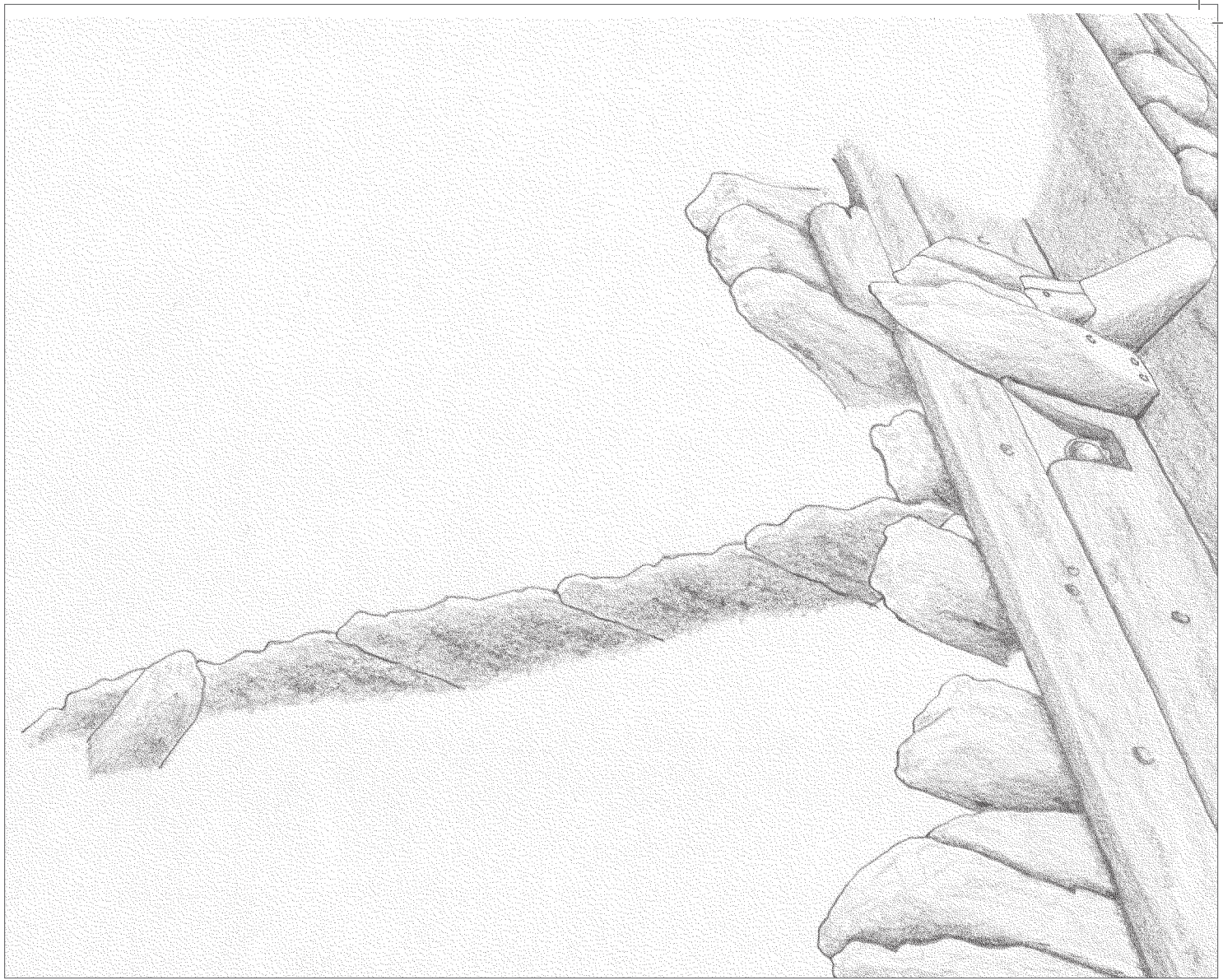
Figure 9.12 Sketch of the deck and bulkhead remains excavated at the stern. Note the recess in the waterway for the scupper (drawing C. Murray).
