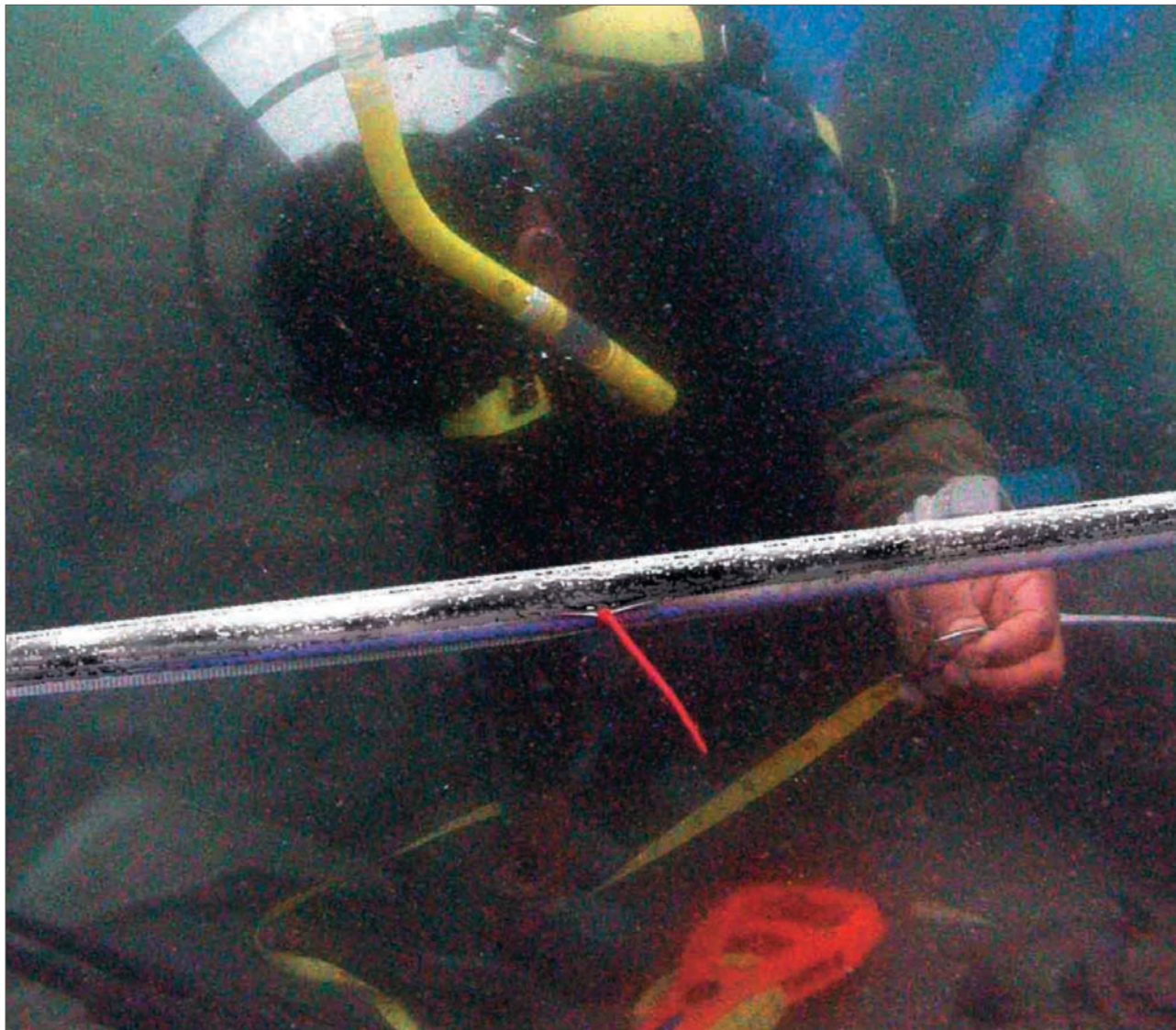
Figure 8.20 Taking measurements from levelled aluminium pole
