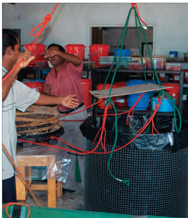
Figure 11.5 Pulley system for handling the barrel
