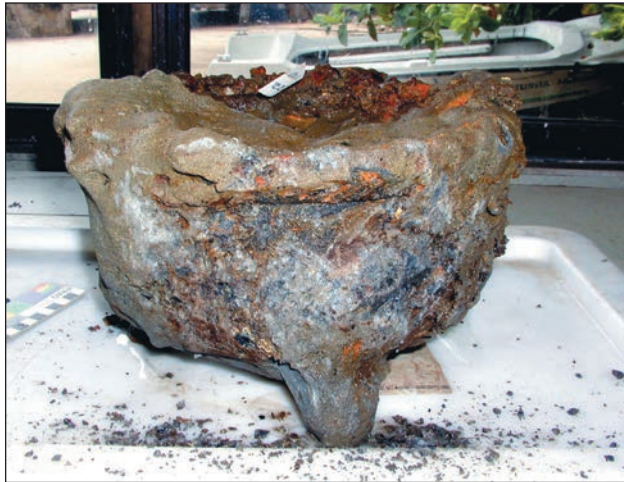
Figure 4.36 : A cast iron cauldron corroded beyond recognition after 350 years under water.
